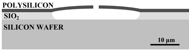
Fig. 2. Bisection of the polysilicon shell-type micromechanical resonator.
