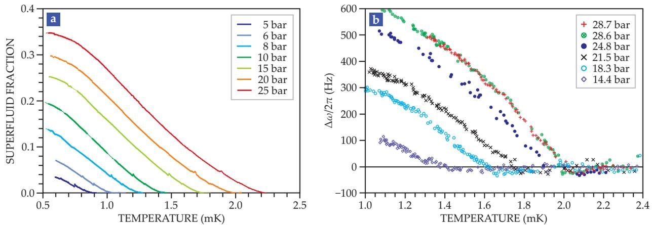
**FIGURE 4. SUPERFLUIDS IN AEROGELS** make themselves known. **(a)** The superfluid fraction is a function of temperature and pressure, as determined by torsional-oscillator experiments.<sup>3</sup> **(b)** The NMR frequency shift  $\Delta\omega$  away from the value for a normal fluid is also a function of temperature and pressure.<sup>4</sup> Note the sharply defined onset of the superfluidity in the measurements, both of which were conducted with a 98% porous silica aerogel.
