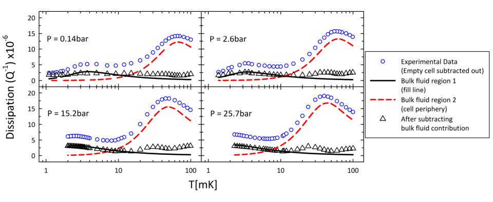
After subtracting bulk:Temperature independent dissipation ~ 2.5x10<sup>-6</sup>
