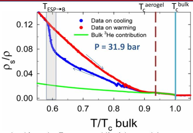
Determined from the Frequency shift of the pendulum.
