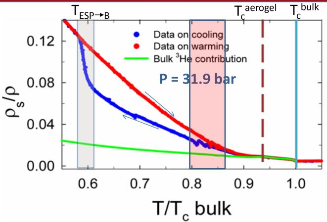
Determined from the Frequency shift of the pendulum.
