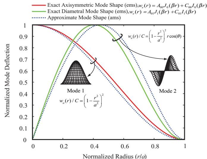
**Figure 2.** Normalized circular and diametral mode shape of a clamped solid circular plate.
