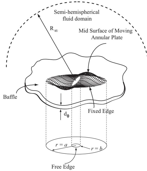
**Figure 1.** Schematic of semi-hemispherical fluid domain above the vibrating annular plate.
