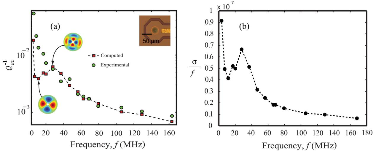
**Figure 3.** (a) Acoustic quality factor computed for experimental measurement carried out on a circular region as shown in SEM picture; (b) Acoustic radiation efficiency as a function of modal frequencies.
