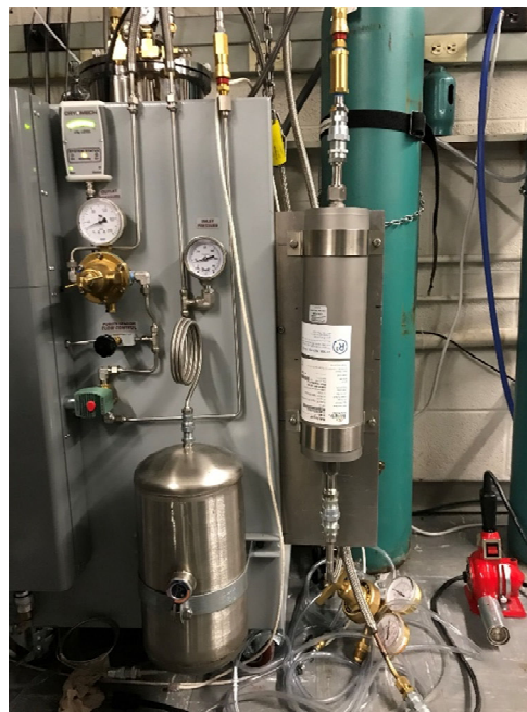
Fig 6 Image of the hydrogen getter panel attached to purifier
