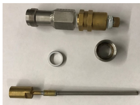
Fig 7. Top image is of the transfer stick end that we capped off and now use a Teflon O-ring to seal. The bottom piece mates with our transfer stick extension. It is only used during the initial transfer.
