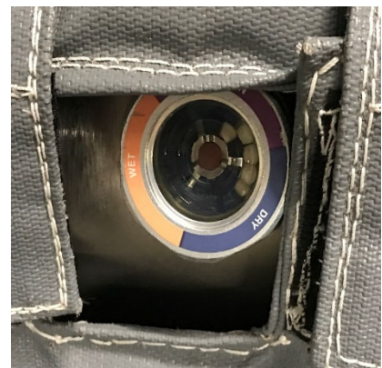
Fig 2 Image of water trap in heater jacket showing lilac colored “dot”.
