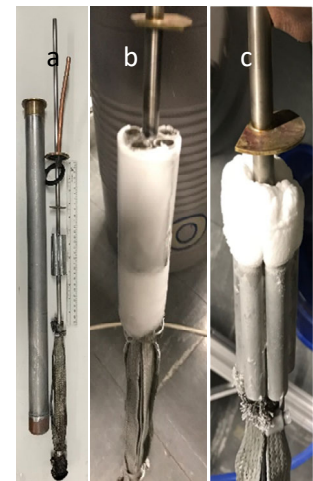
Fig 3 a) Liquid nitrogen trap to condense water b) with ~200 gm extracted c) remaining 50 gm trapped.
