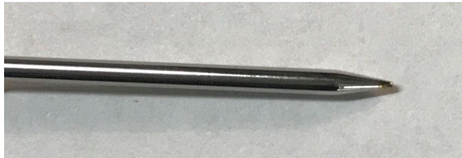
Fig 1 Shows discoloration at the tip of discharge electrode.
